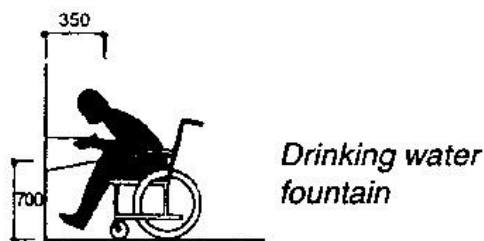
Figure 3: Indicative placement of drinking water facility for differently-abled
