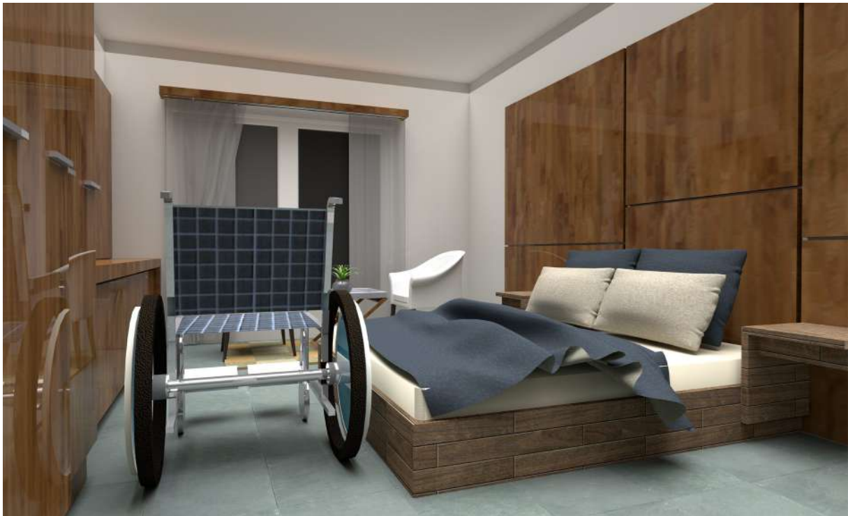
Figure 6.5 Universally Accessible Guest Room With Clear Route to the Bed
